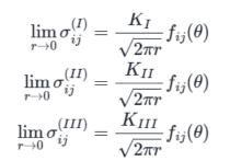
When encountering a problem of mixed-mode, we can use superposition to find the stresses at the crack tip such that :
