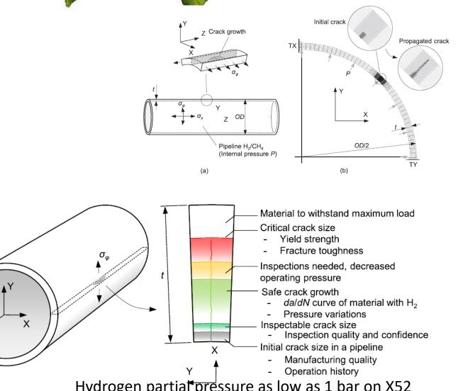
Hydrogen partial pressure as low as 1 bar on X52 will degrade the material.
