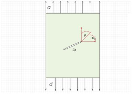
We can use superposition and obtain the crack tip fields as
