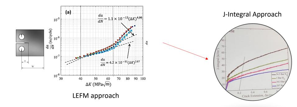
ASME B31.12 features a nonlinear correlation (in logscale) between crack growth rate and SIF range. ASME B31.12 suggests a characteristic design da/dN curve for hydrogen pressure under 20 MPa (200 bar).
