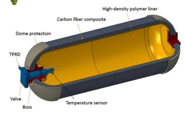
Design of hydrogen storage tanks under fatigue and vibration condition
